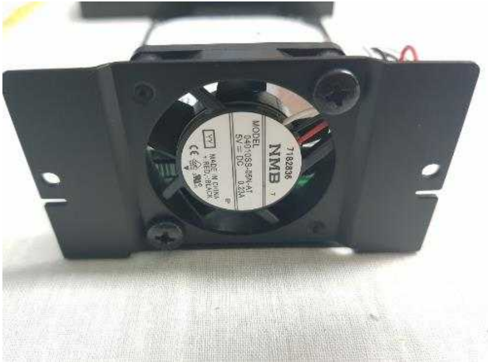
< DC fan view in HDD slot >
