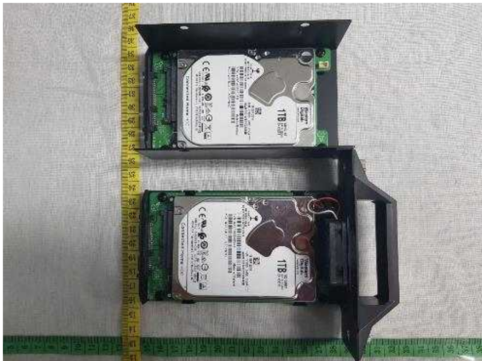
< Internal view of HDD slot >
