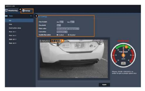
Make note of the dial position as the pointer moves through the dial. Ideally you should target the vehicle to be at the center of the image, well zoomed in as in the above picture.
