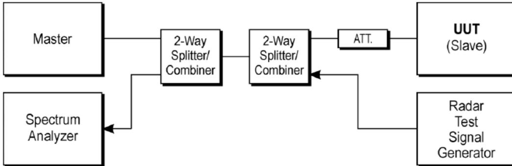
**Figure 5: Set-up B**
