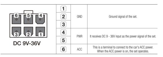
• If the ACC yellow line on the power cable is not connected to the power or the car's ACC terminal, the power will not turn on.
